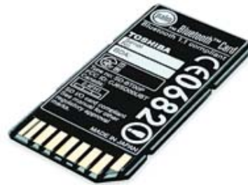
A Bluetooth card can add short-range wireless connectivity to a PDA.
