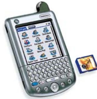
[Photo: PalmSource] Extra memory and other features often can be added to a handheld through small add-on cards.
